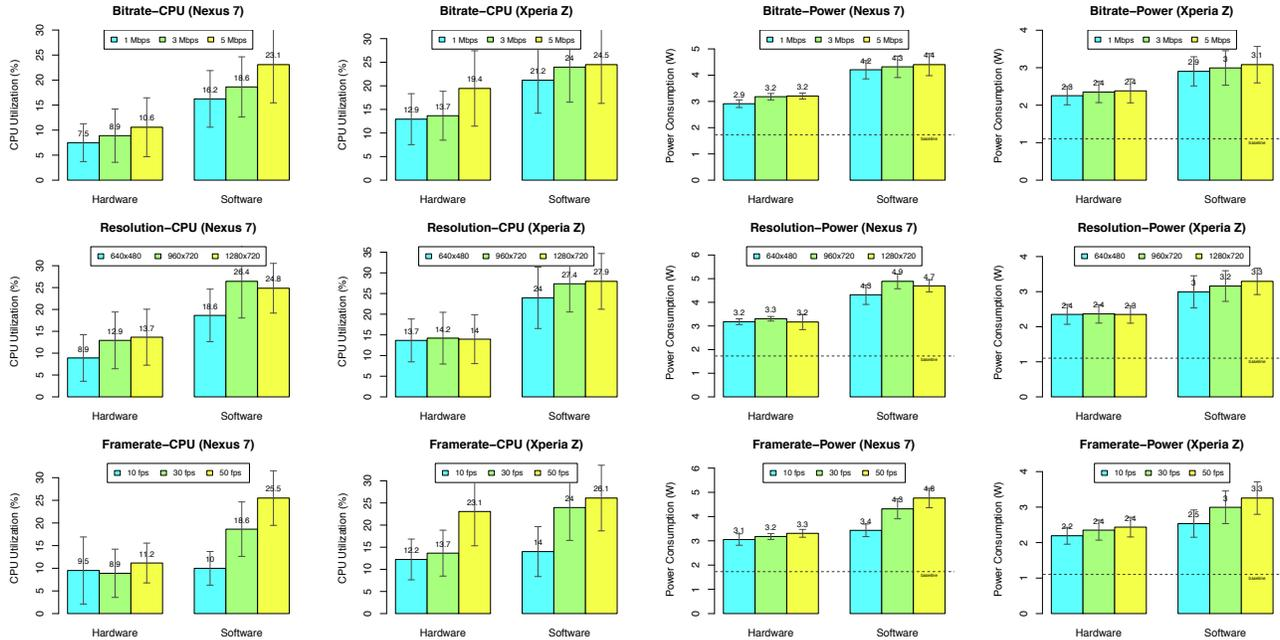
Fig. 3. Measured CPU utilization and power consumption under various codec parameters.
