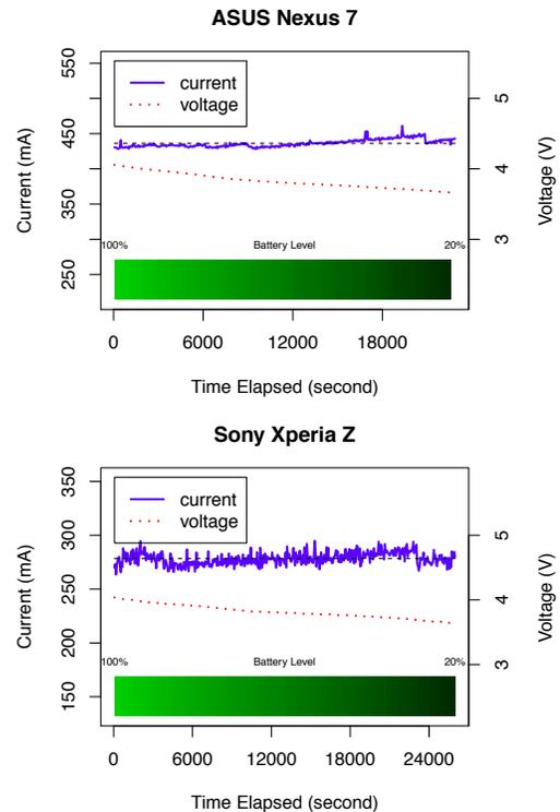
Fig. 2. The voltage and current levels measured under the baseline configuration.
